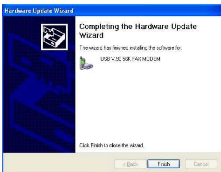
10. To verify if the device is enabled in your system, make sure the device name is modified to be **USB V. 90 56K Fax MODEM**. If not, consult your distributor for technical support.
